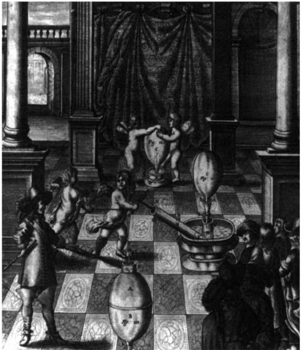
Otto von Guericke's first pump demonstrated before witnesses. From Schott's Mechanica hydraulico-pneumatica (Wurzburg, 1657), p. 445.
